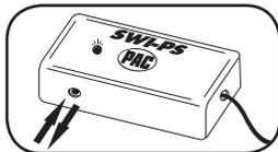
Press and release the programming/mode button on the SWI-PS.
