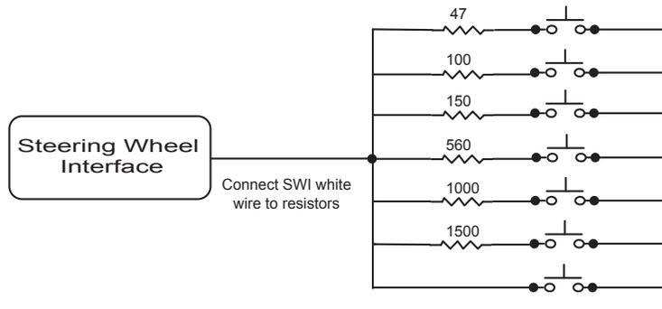
By putting two or more resistor in series, you can come up with additional values. Ex.  $150 + 1000 + 1500 = 2650\text{ohms}$ .
