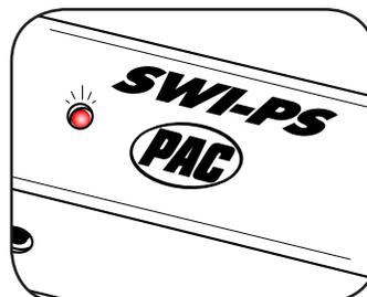
Once programming is completed, wait 7 seconds. The LED will flash three times indicating end of programming. The Interface will then flash the version number it was programmed for.
