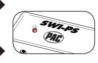
In either case, the LED will flash once and stay on. Skip to Step 20. You have 7 seconds to perform the next step.
